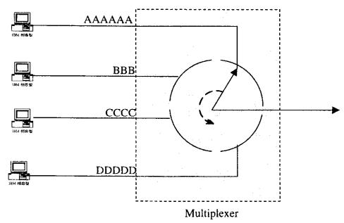
In above figure, the switch is rotating counter clockwise. As we interleave the various transmissions by character (equal to one byte each) from each computer station (the data are shown in each computer station), please show the final data stream from the multiplexer output. (5%)
